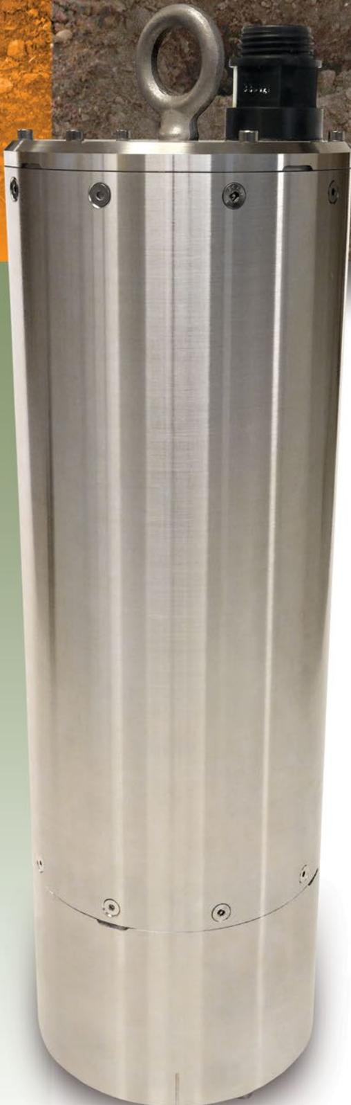
The **Trillium Posthole Seismometer** is a very broadband seismometer designed for down-hole deployments. The instrument is housed in a stainless steel enclosure incorporating a high-pressure, marine-grade connector making it suitable for uncased buried/posthole installations. An advanced leveling system allows the instrument to self-correct over a tilt range of  $\pm 5$  degrees ( $\pm 10$  degrees optional).
