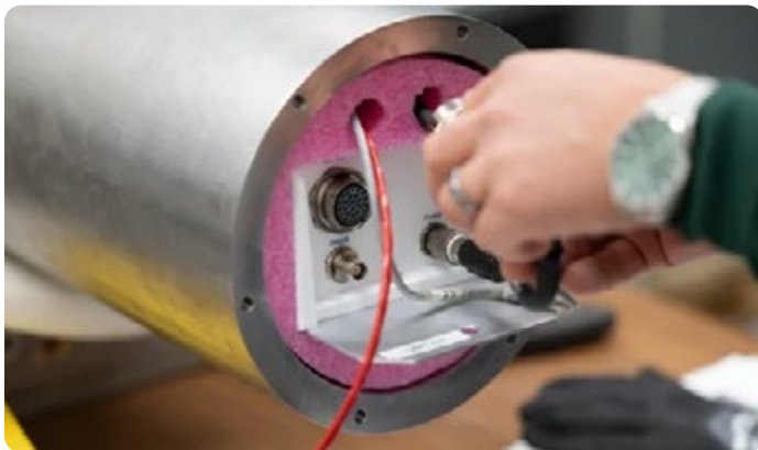
Rob Anthony puts in the Seismometer Interface Module while assembling a seismometer at the Physical Sciences Laboratory in Stoughton, Wisconsin on Aug. 7, 2025. Photo courtesy of Taylor Wolfram / UW-Madison
