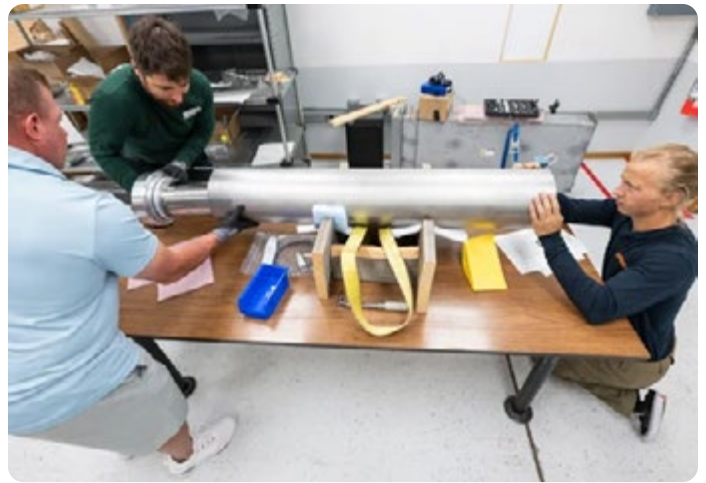
Jason Patton, Rob Anthony, and Skyler Grulke slide a part into the pressure vessel tube while assembling a seismometer at the Physical Sciences Laboratory in Stoughton, Wisconsin on Aug. 7, 2025. Photo courtesy of Taylor Wolfram / UW-Madison
