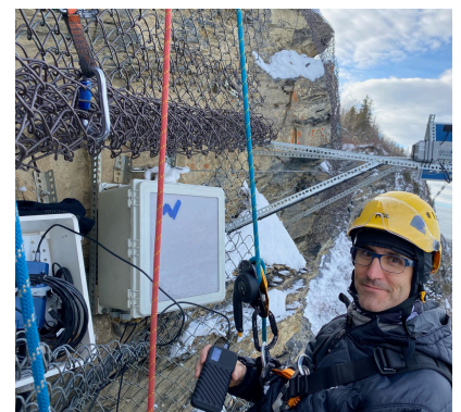
Prof Bernard Giroux from the Institut national de la recherche scientifique (INRS) is shown holding a Portable Harvester connected to a Pegasus Digitizer.
