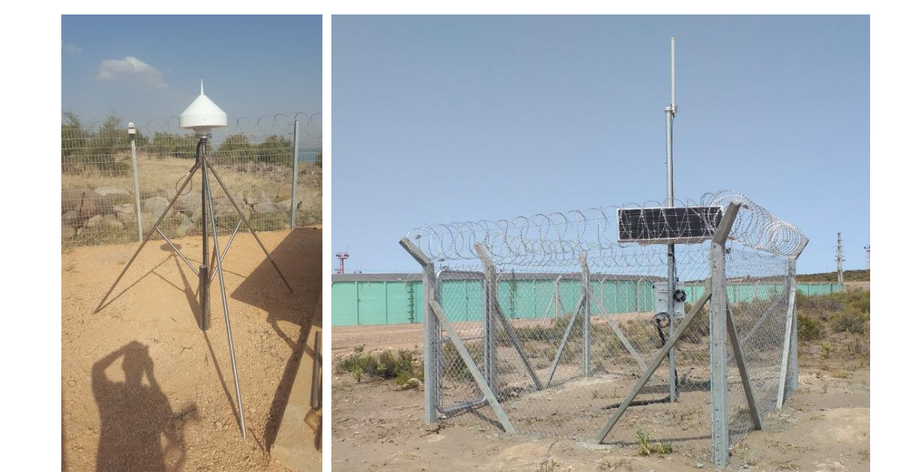
An Alaska Volcano Observatory Infrasonic sensor under shielding (foreground) at site GASW, Gareloi Volcano, Andreanof Islands, western Aleutians. Acoustic and Seismo-Acoustic stations throughout the observatory take advantage of the low-power, robustness and reliability of Centaur. Photo: Boyce, Ellie Image courtesy of the AVO/UAF-GI.
