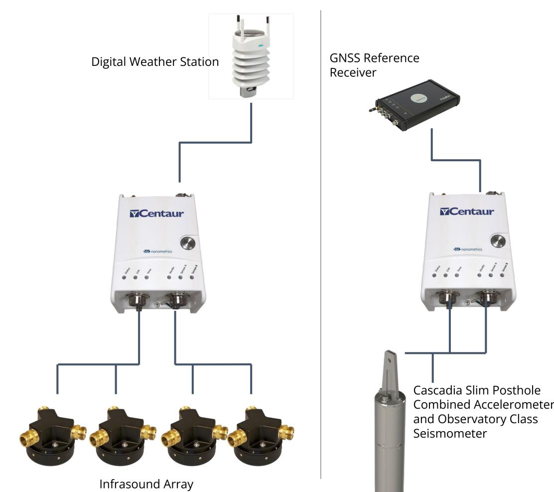
Centaur, Trillium, Titan and Cascadia by Nanometrics Inc. WTX536 Digital Weather stations by Vaisala PolaRx5 GNSS Reference receiver by Septentrio Model 64 Infrasound sensor by Chaparral Physics
