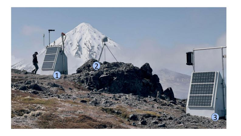
Shallow-braced GNSS monument using Centaur automatic backfill features with a Septentrio PolaRx5 GNSS Reference receiver. These features allow automatic recovery of data after service interruptions and tracking of complete acquisition metrics including latency monitoring. Photos: Laporte, Michael Image courtesy of Nanometrics
