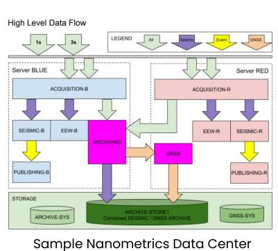
Architecture with Redundant Processing Toolchains
