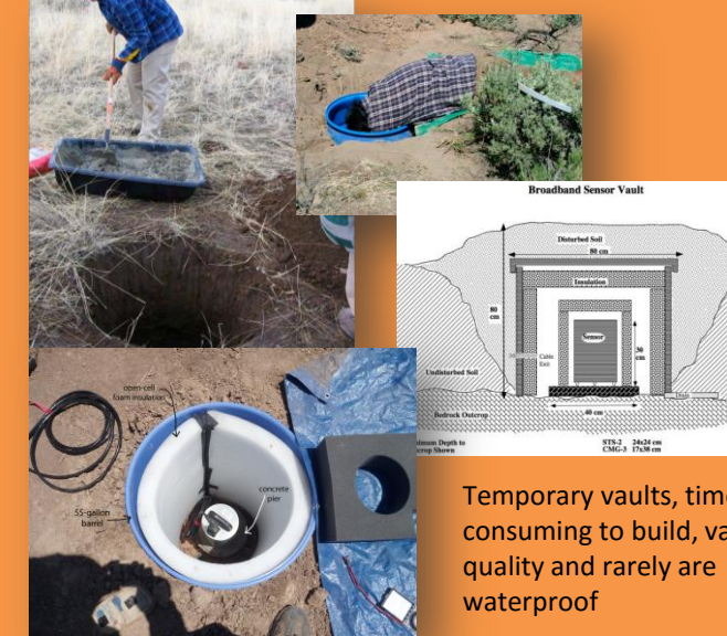
Blue cylinder is improvised pressure case for pier instrument
