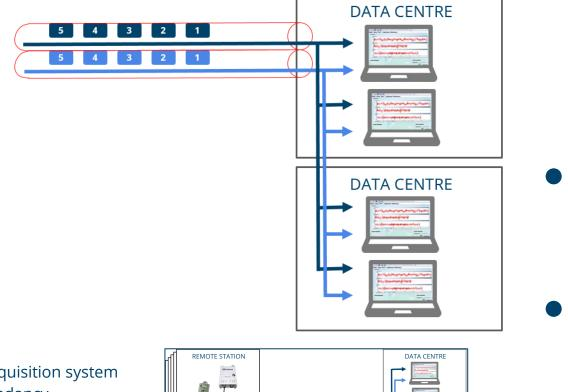
Abstract view of the TRUAA acquisition system architecture, meeting all redundancy requirements while minimizing operational cost (bandwidth).
