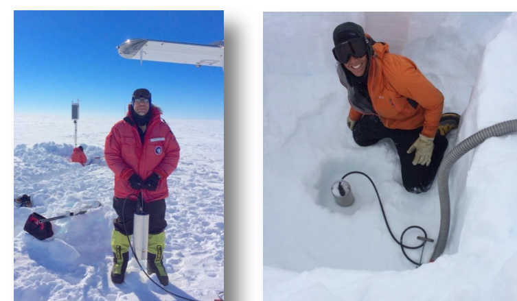
Rick Aster on left and Doug Bloomquist on right deploying T120PHQ sensors during the Ross Ice Shelf Experiments
