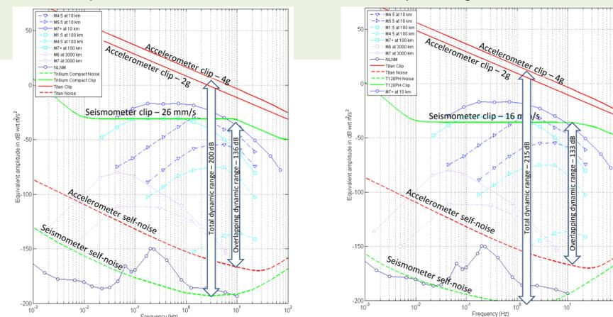
Two examples are shown: a Titan 4g accelerometer combined with a Trillium Compact 120s seismometer, and the same accelerometer with a Trillium 120 Posthole. Other options can be considered, e.g.: GSN-class 360s seismometers, configuring the accelerometer to 2g.
