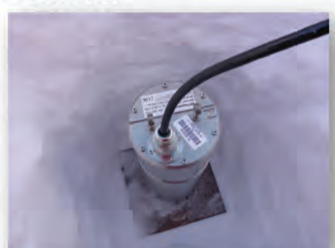
Fully integrated portable broadband/digitizer system deployed at the South Pole, Antarctica, photo courtesy IRIS PASSCAL Instrument Center
