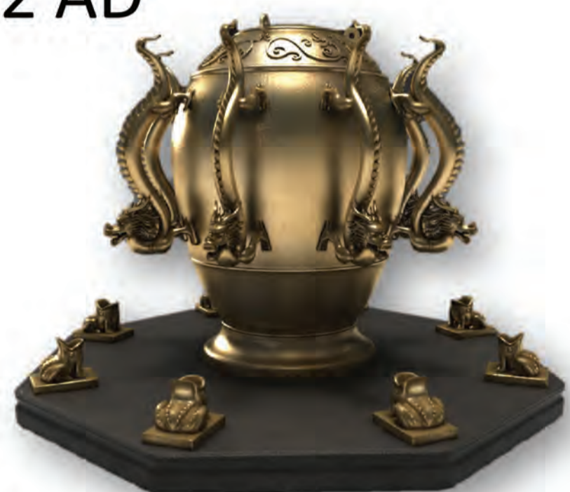
Photo by Houfeng Didong of modern replica of Zhang Heng's seismoscope
