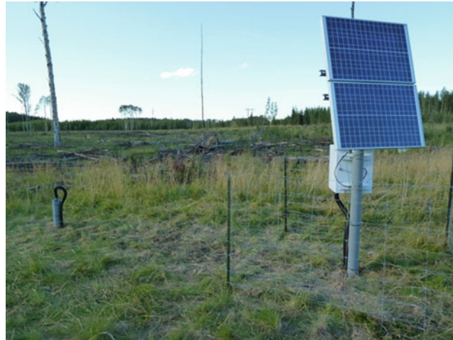
Fig. 6 Rural posthole installation with cellular communications in Alberta, Canada
