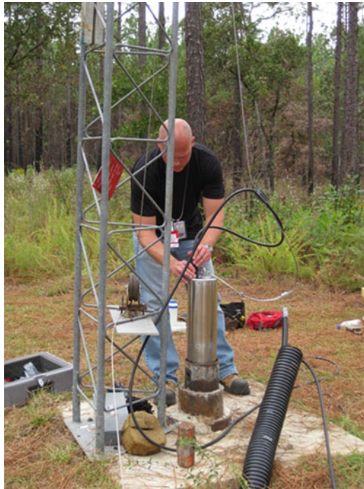
Fig. 9 Rural borehole seismometer deployment in Alberta, Canada
