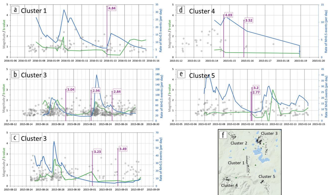
**Figure 7.** (a–e) Temporal variation of magnitude, *b*-value, and seismicity rate for five different time windows around major events. (f) Map shows the location of the recorded events over the past two years near Crooked Lake, Alberta.
