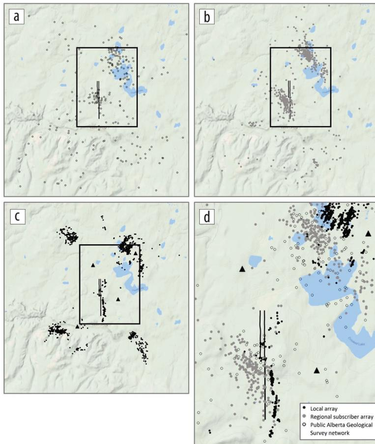
**Figure 3.** Network performance comparison using a data set recorded near an active target HF pad in the Duvernay region of central Alberta. (a) AGS network catalog. (b) Regional subscriber array catalog. (c) Local four-station array catalog. (d) Closer view of overlapping three-event catalogs adjacent to the well pad.
