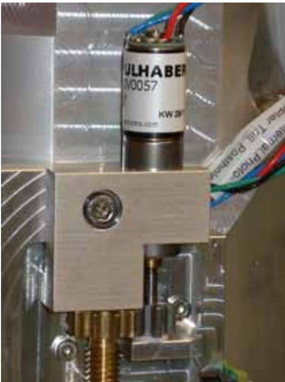
Figure 2. The leveling mechanism integrates a high-torque-density stepper motor and a gearbox to adjust the position of the instrument. (Courtesy of Nanometrics Inc.)
