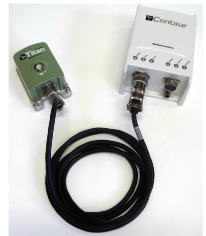
Titan accelerometer connected to and powered by a Centaur digitizer
